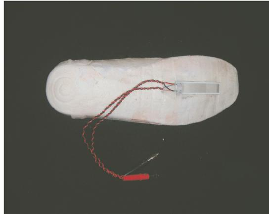
Figure 3.2: Position of the symmetric heterogeneous bimorph in the shoe.
