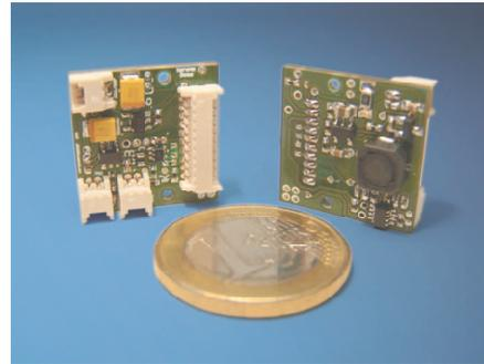
**Figure 5. The PCB prototype of the power management unit.**
