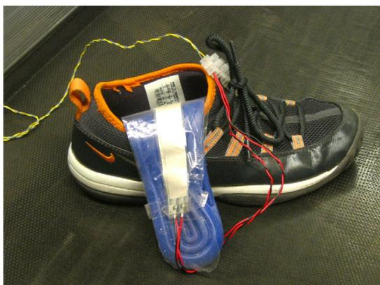
Fig. 2. Prototype of the piezoelectric film inserted in shoe. There are two DT4-028K/L piezoelectric films from MSIUSA in parallel inside the shoe.
